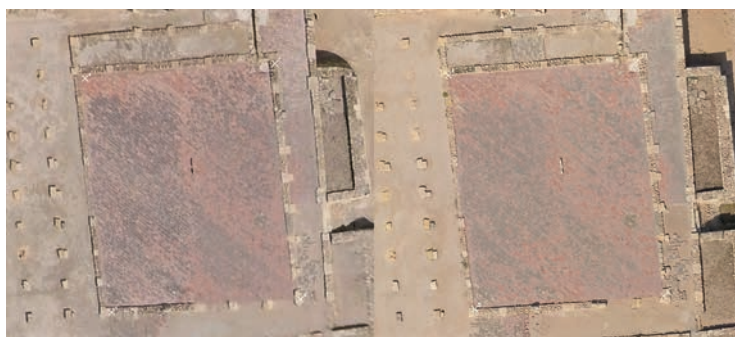
Fig. 3b. The Great Mosque. Comparison between the photogrammetry carried out in 2011 (left) with that of 2021 (right). In this latter, in addition to the increase in definition, it is possible to see the increase in accuracy with the topographic control points coinciding with the corners of the Mosque's courtyard.
